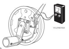
The threshold voltage of a controller is the voltage applied to
