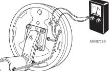
at a time. If the high amperage reading drops to zero by unplugging the trailer, then the short is in the trailer. If the amperage reading remains high with all the brake magnets disconnected, the short is in the trailer wiring.
