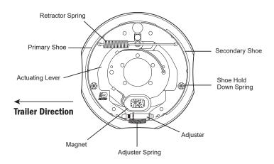
When the electrical current is fed into the system by the controller, it flows through the electromagnets in the brakes. The high capacity electromagnets are energized and are attracted to the rotating armature surface of the drums which moves the actuating levers in the direction that the drums are turning.
