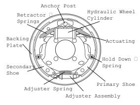
leave the anchor and causes the primary shoe to move against the anchor. Action of the brake is the same in reverse as forward.
