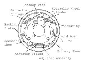
through the adjuster assembly. Braking in reverse is significantly less effective than in the forward direction.
